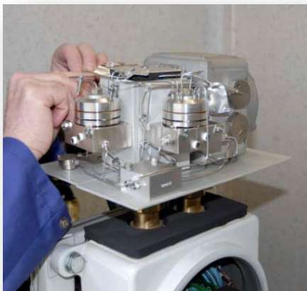
The above photograph shows the instrument undergoing a chromatographic valve upgrade. Two of the three 6-port chromatographic valves can be seen. The sample shut off valve is the rectangular device mounted on the plate in the centre.
